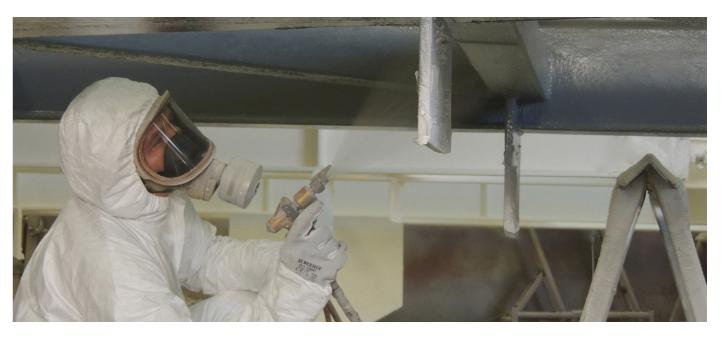
Alternatively, E&L Enterprises also provides the innovative Powder Coating finishing process which involves the application of a dry powder through heat. Powder coating allows for a sturdy, durable finish. The client can choose from a variety of texture and colour finishes.
